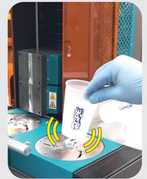
Container automatic detection sensors
