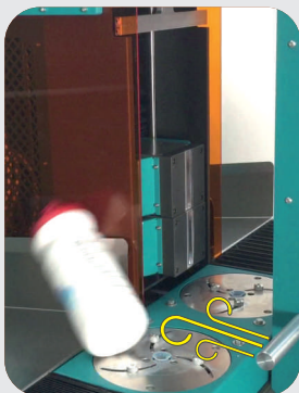
Automatic unloading with integrated blow
