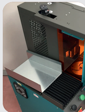
Unloading slides for direct packaging
